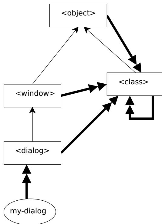
Figure 4.1: Example inheritance hierarchy for simple classes.
