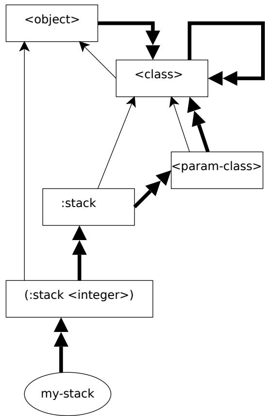
Figure 4.2: Example inheritance hierarchy for parametrized classes.
