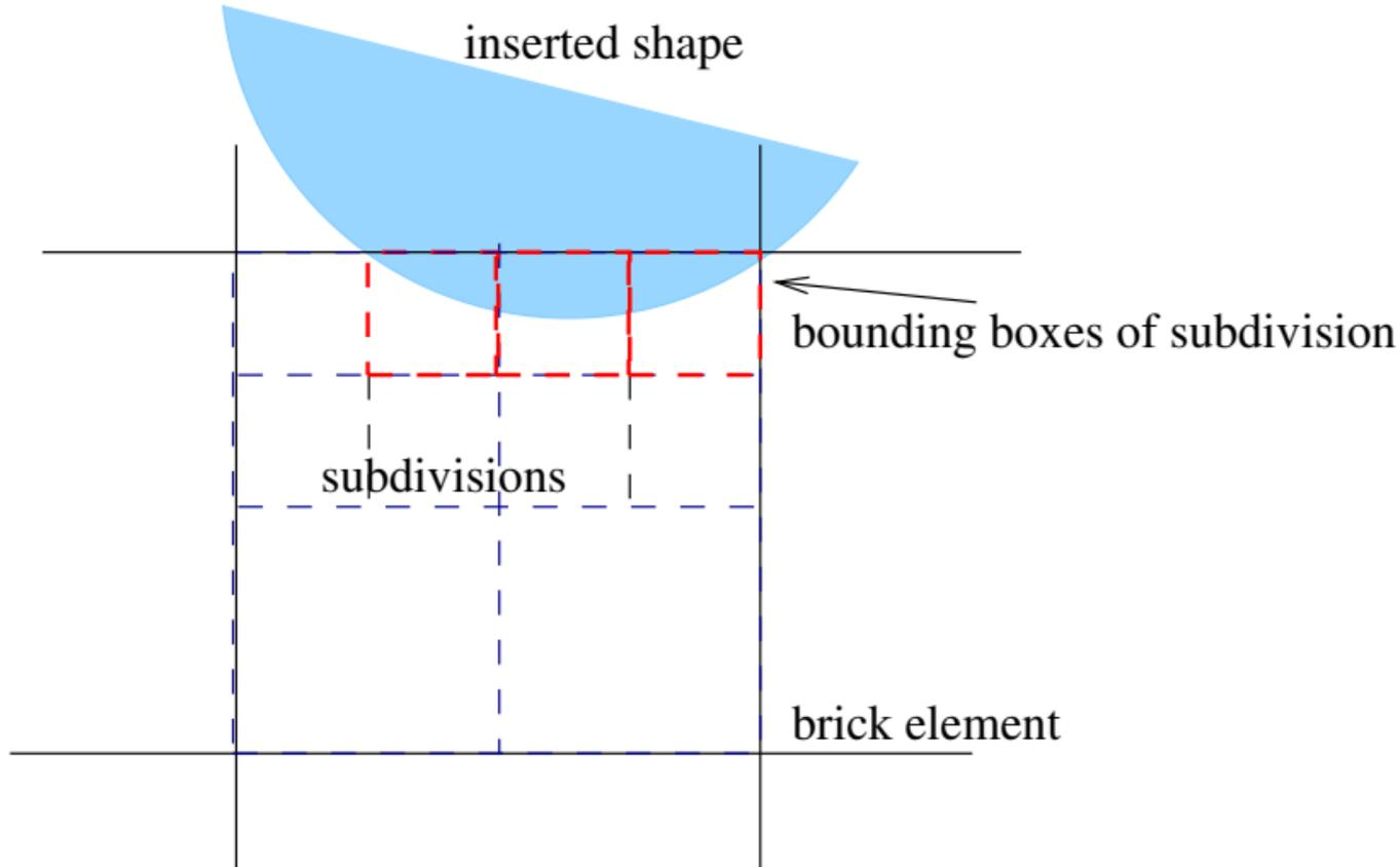
Brick or Hex Diatom Algorithm Bounding Box on Brick Element
